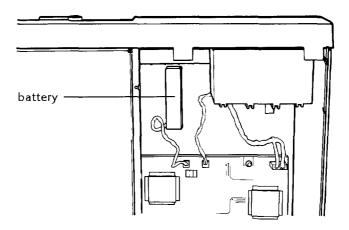
To disconnect the battery from the main system board, pull up on the connector plugged into socket CN1, as shown below.
